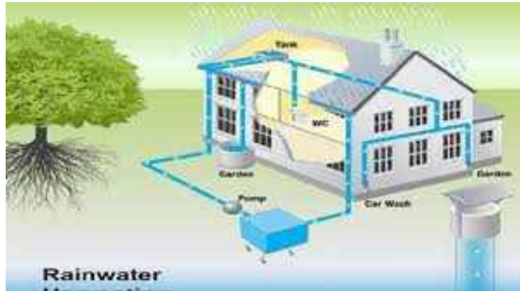
Fig.1 Rainwater Harvesting System
